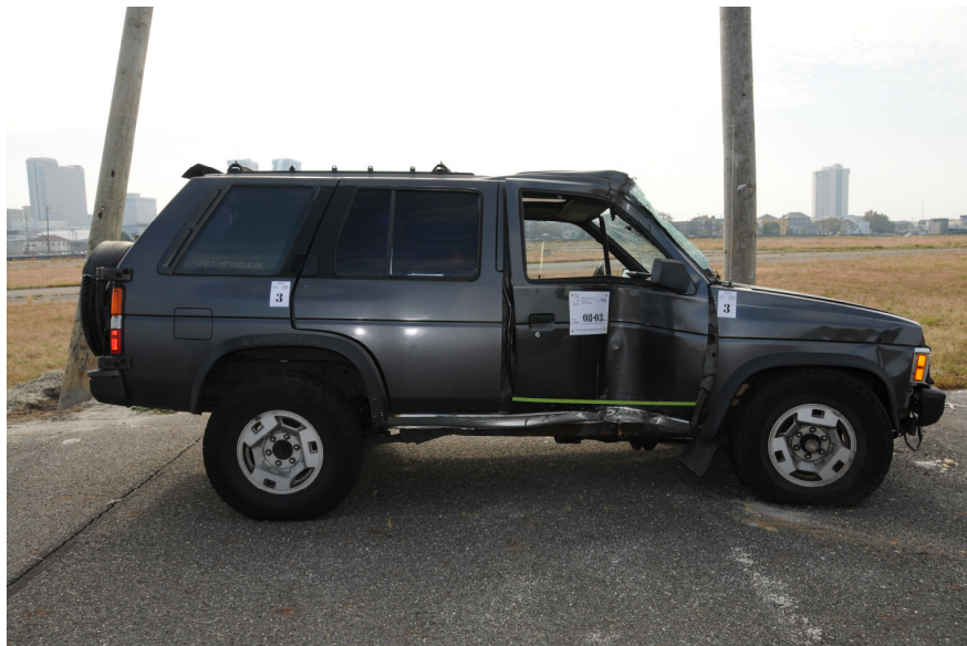
Photograph 5: Test 3--Damaged Nissan (KEES = 22.5 mi/hr)
