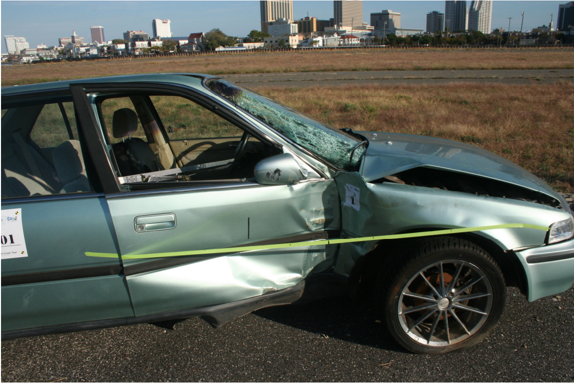
Photograph 3: Test 1--Damaged Honda (KEES = 21.0 mi/hr) and Masking Tape Used for Crush Measurements
