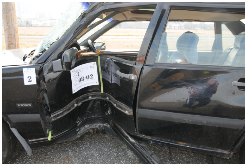
Photograph 4: Test 2--Damaged Volvo (KEES = 22.5 mi/hr)
