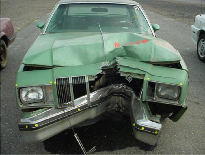
Photo 1 – Results from Joint Conference 2003 crash tests. Oldsmobile impact speed: 28 mi/hr. Maximum crush = 25.2 inches.
