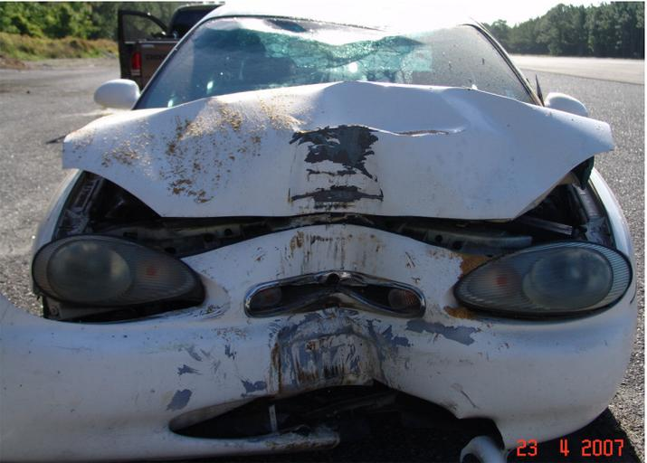
Photo 5 – Results from IPTM Special Problems 2007 test. 1999 Mercury Sable. Impact speed 43 to 43 mi/hr. Maximum crush = 14.75 inches. Photo by Sergeant Greg Waters, N.Z Police: Serious Crash Unit (Waikato).
