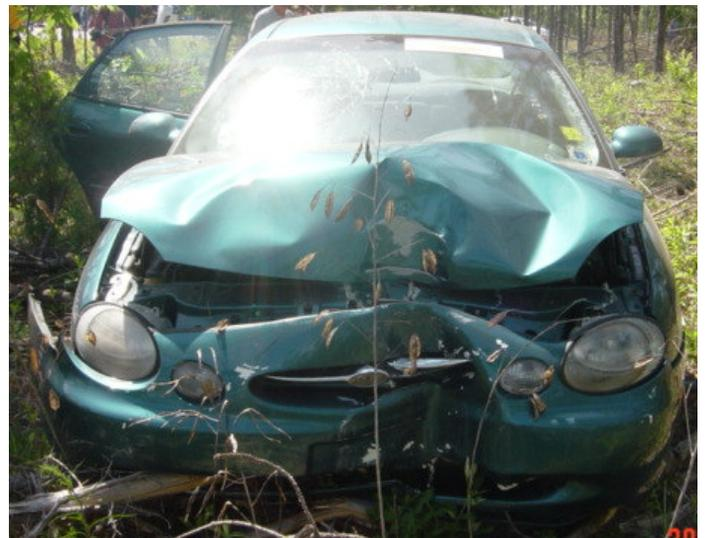
Photo 4 – Results from IPTM Special Problems 2007 test. 1998 Ford Taurus. Impact speed 48 to 49 mi/hr. Maximum crush = 15.50 inches. Photo by Sergeant Greg Waters, N.Z Police: Serious Crash Unit (Waikato).
