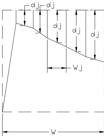
Figure 1 (Idealized crush mechanism—from Wood, SAE 930894)
