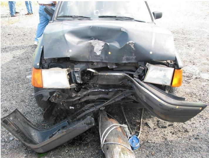
Photo 3 – Results from Joint Conference 2003 crash tests. Ford Impact speed = 29 mi/hr. Maximum crush = 16.8 inches.
