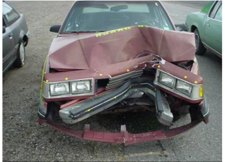
Photo 2 – Results from Joint Conference 2003 crash tests. Chevrolet impact speed = 30.5 mi/hr. Maximum crush = 21.6 inches.
