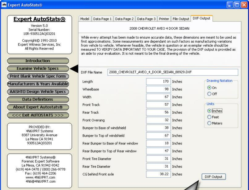
For DXF output, the default settings (as of June 2010) are INCHES and WITH Text.
