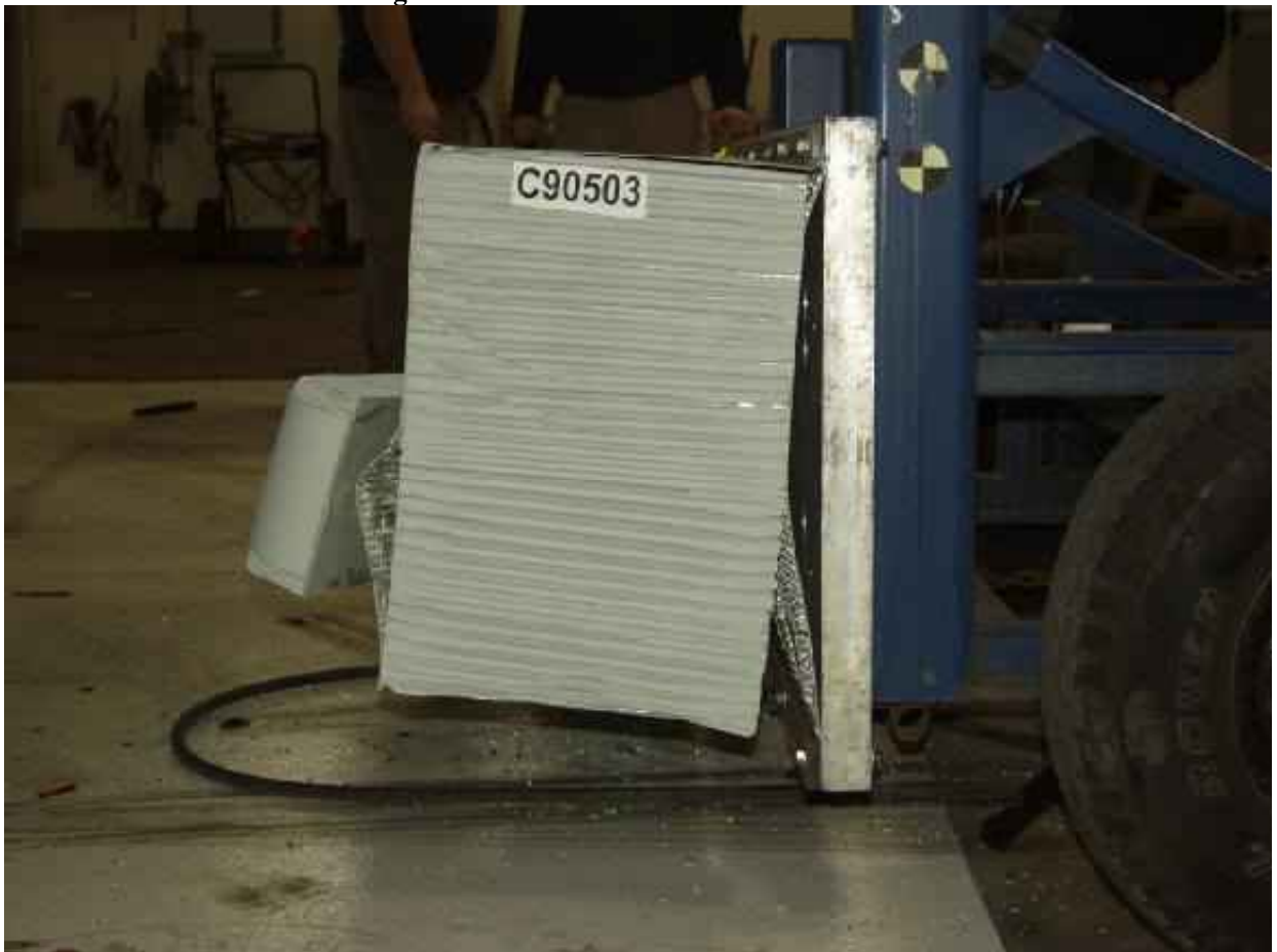
Figure A-22: Post-Test MDB Left Side View
