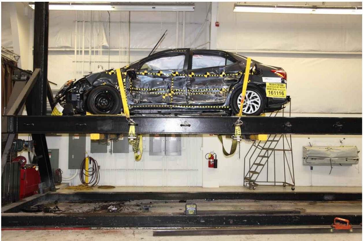
100 FMVSS No. 301 Static Rollover 360 Degrees
