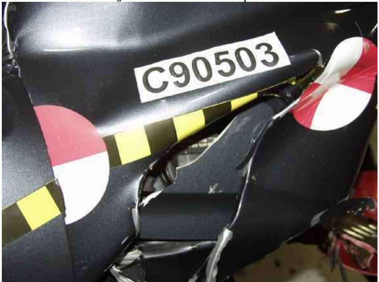
Figure A-36: Post-Test Fuel Filler Cap View
