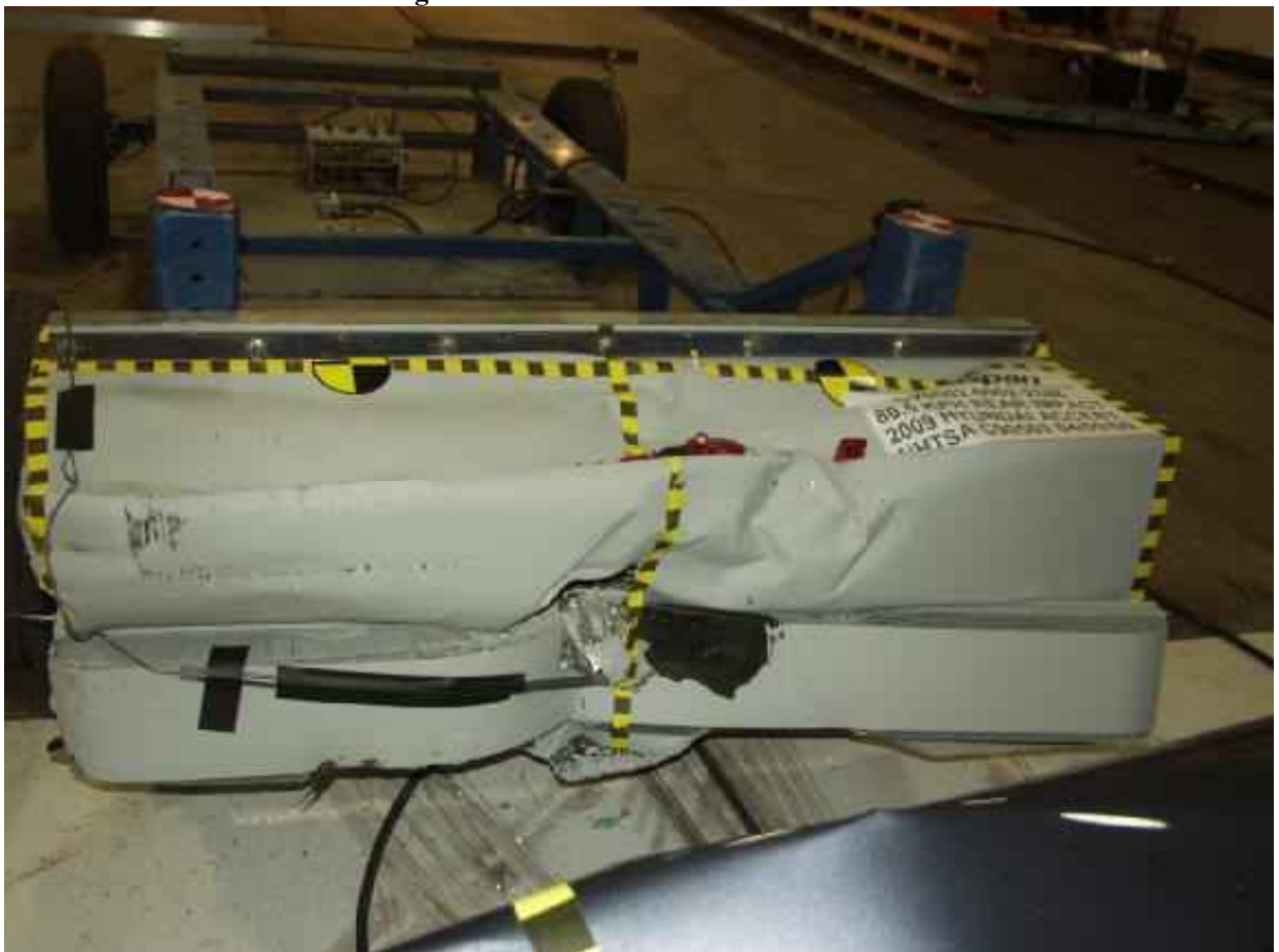
Figure A-20: Post-Test MDB Front View
