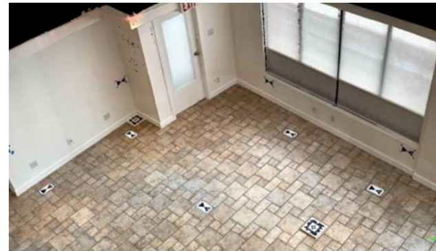
FIGURE 4: Recon-3D data in CloudCompare software showing an example scene with measurement markers and AprilTags.
