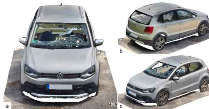
Fig. 5. Screenshots of the 3D point cloud from the parked car. Views of the car from different angles are given in images a – c. The license plate has been painted over to hide the original license plate number. The point size of the data points was increased to provide a better visualization of the data.
