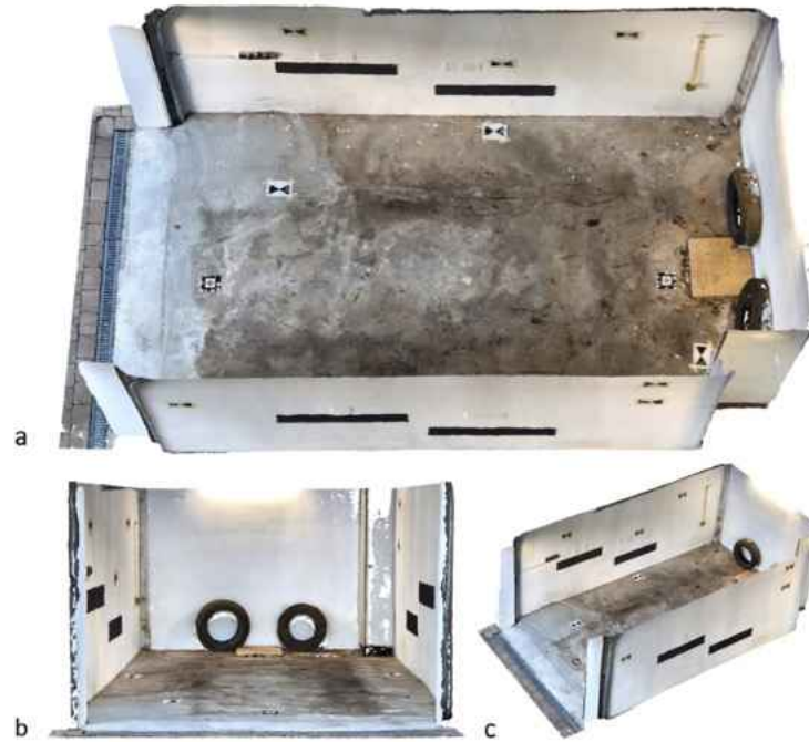
Fig. 4. Screenshots of the 3D point cloud from the garage. Views of the scene from different angles are given in images a – c. The point size of the data points was increased to provide a better visualization of the data.
